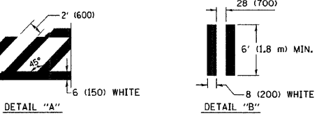
TYPICAL CROSSWALK MARKING
