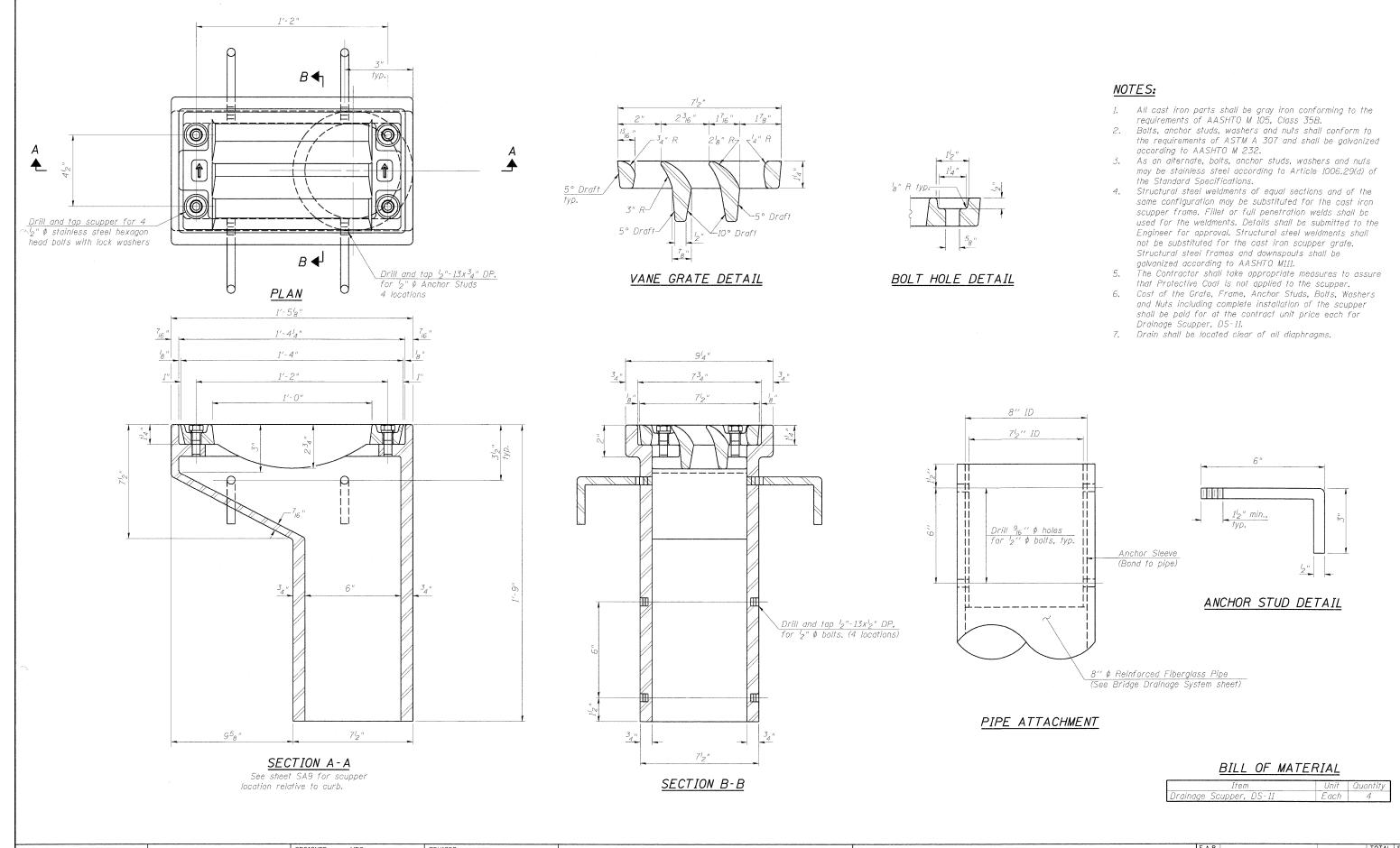
TOTAL SHEET NO. DESIGNED MBQ REVISED SECTION DRAINAGE SCUPPER, DS-11 STATE OF ILLINOIS REVISED DRAWN мва F.A.P. 392 FRANKLIN CONNECTOR (AT 26th STREET) 392 1717-2-3B-R COOK **JACOBS** CHECKED JRW REVISED **DEPARTMENT OF TRANSPORTATION** STRUCTURE NO. 016-1064 CONTRACT NO. 62197 PLOT DATE = 1/12/2009 DATE SHEET NO. SA15 OF SA31 SHEETS STA. 11+81.01 1/13/09 REVISED SCALE: NTS FED. ROAD DIST. NO. 7 | ILLINOIS FED. AID PROJECT
