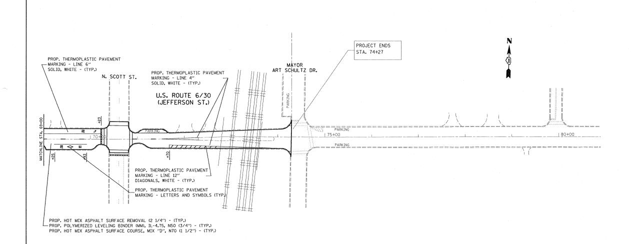
NOTES: LIMIT OF RESURFACING ON SIDE-STREETS THROUGH OUT THE IMPROVEMENT SHALL BE TO THE RADIUS OF RETURN OR AS DIRECTED BY THE ENGINEER.
