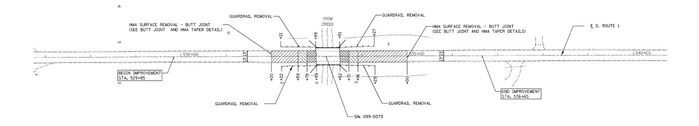
NOTE: THE EXISTING PAVEMENT CONSISTS OF 3 INCHES OF HOT-MIX ASPHALT OVER 9 INCHES OF PCC BASE COURSE
