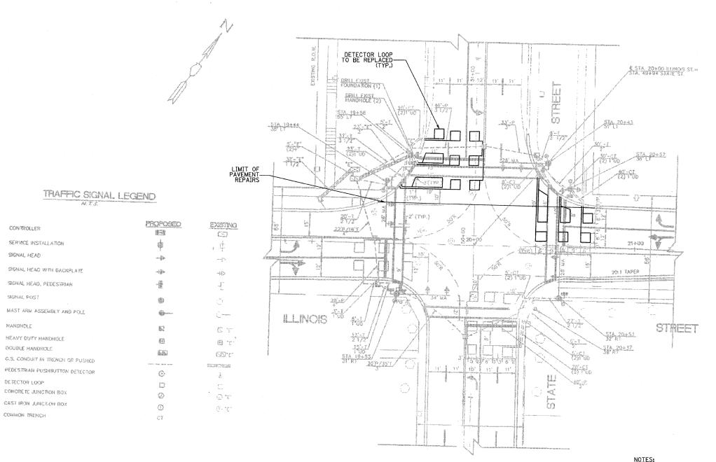
1. THIS PLAN IS FOR THE PURPOSE OF REPLACING DETECTOR LOOPS ONLY. ALL OTHER INFORMATION SHOWN IS NOT RELATED AND SHALL BE DISREGARDED.
