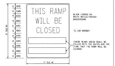
THESE SIGNS ARE REQUIRED ON BOTH SIDES OF THE RAMP, MINIMUM OF 1 WEEK IN ADVANCE OF THE CLOSURE.
