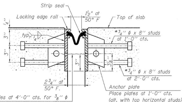
7/16" φ holes at 4'-0" cts. for 3/8" φ bolts. All bolts shall be burned, sawed, or chipped off flush with the plates after forms are removed, typ.
