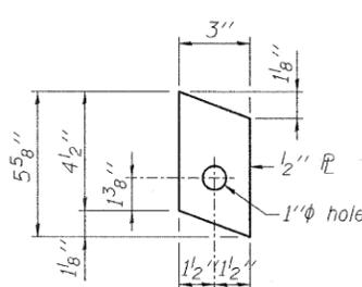
**ANCHOR PLATE (for welded rail)**
