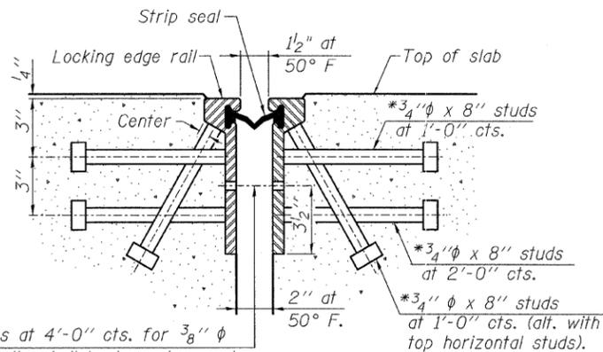
7/16" φ holes at 4'-0" cts. for 3/8" φ bolts. All bolts shall be burned, sawed, or chipped off flush with the plates after forms are removed, typ.
