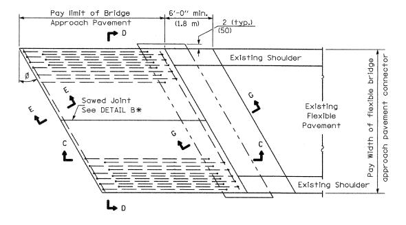
BRIDGE APPROACH PAVEMENT CONNECTOR (FLEXIBLE)
