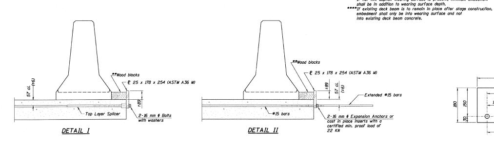
\*\*Wood blocks may be omitted when required to provide minimum stage traffic lane width. When the wood blocks are omitted, the concrete barrier shall be in direct contact with the steel retainer plate.
