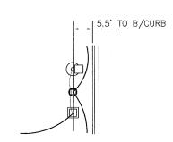
5.5-FT TYPICAL SETBACK DISTANCE FROM BACK OF CURB TO C.L. OF LIGHT POLES, GULF JUNCTION BOXES, AND LIGHTING CONTROL PEDESTALS
