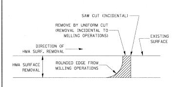
WHEN MILLING OPERATIONS PRODUCE A ROUNDED EDGE, THEN A SAW CUT SHALL BE USED TO MANUFACTURE A PERPENDICULAR EDGE AS SHOWN IN THE DETAIL. THE ENGINEER SHALL BE THE SOLE JUDGE CONCERNING THE USE OF THIS DETAIL
