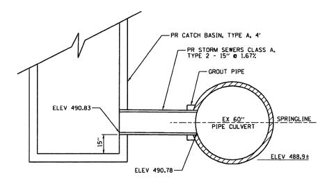
THE CONNECTION TO THE EXISTING CULVERT WILL BE INCLUDED IN THE UNIT PRICE FOR THE PROPOSED PIPE INSTALLED. THE UNIT PRICE SHALL INCLUDE CORE DRILLING THE EXISTING CULVERT WALL, GROUTING THE PROPOSED PIPE IN PLACE AND ALL OTHER RELATED WORK AS DETAILED HEREIN.
