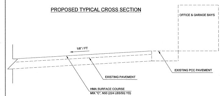
NOTES: TO MAINTAIN THE 1/8"/FT SLOPE THE PARKING LOT SHALL BE PAVED IN A DIRECTION THAT RUNS PARALLEL WITH THE GARAGE AND OFFICE.
