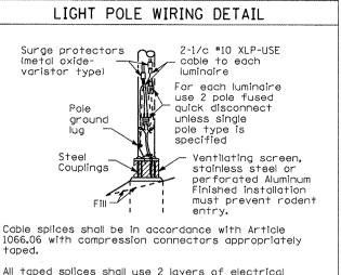
All taped splices shall use 2 layers of electrical tape over 3 layers of rubber tape as required by the Standard Specifications. Coat the finished taped splice with bonding compound.
