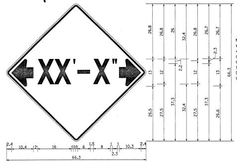
W12-2 - Horizontal Clearance Sign 48.0" across sides, 1.9" Radius. 0.8" Border, 0.5" Indent, Black on Orange; Standard Arrow Custom 10.4" X 8.1" 180° Black 11 Inch D Series Lettering; Standard Arrow Custom 10.4" X 8.1" 0°
