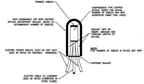
SPLICING ELECTRIC CABLES **BASIC MATERIALS AND METHODS**
