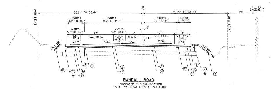
\* PROPOSED CURB AND GUTTER SHALL HAVE A MINIMUM THICKNESS OF (9) INCHES ACCORDING THE IDOT STD. 606001. PROPOSED CURB AND GUTTER WITH A THICKNESS GREATER THAN (9) INCHES WILL NOT INCLUDE ADDITIONAL PAYMENT.
