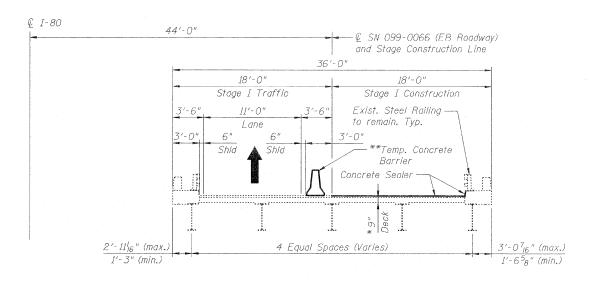
\*  $6\frac{1}{4}$ " reinforced concrete slab with  $2\frac{3}{4}$ " Latex Concrete Overlay
