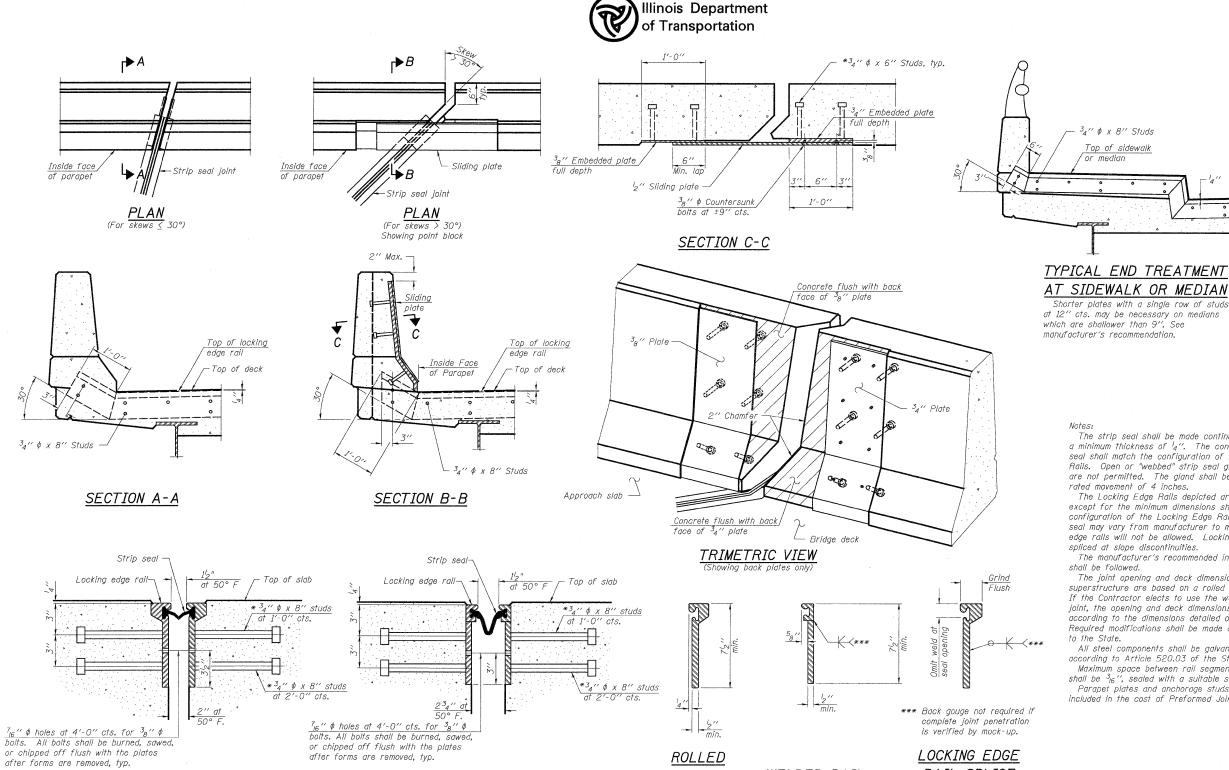
SECTION THRU ROLLED RAIL JOINT
