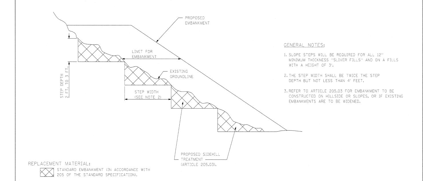
...\D446158-sht-detail SLOPE DETAILS.dgn 12/16/2010 1:23:26 PM
