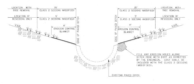
NOTES: THIS WORK SHALL BE PAID FOR AT THE CONTRACT UNIT PRICE PER ACRE FOR CLASS 2 SEEDING (MODIFIED), AND PER SQ. YD. FOR EROSION CONTROL BLANKET, WHICH PRICE SHALL INCLUDE ALL MATERIAL, LABOR AND EQUIPMENT TO COMPLETE THE WORK IN PLACE AS SHOWN.
