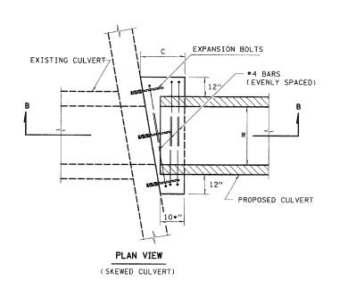
ILLINOIS DEPARTMENT OF TRANSPORTATION **CONCRETE COLLAR DETAIL** FOR BOX CULVERT EXTENSIONS
