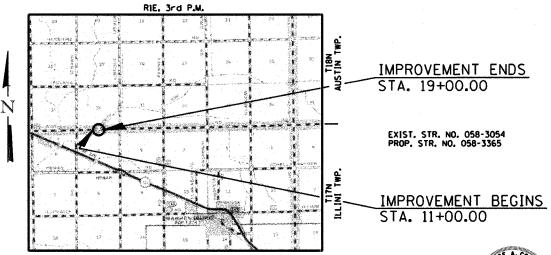
IMPROVEMENT CONSISTS OF THE REMOVAL OF A SINGLE SPAN STEEL PONY TRUSS BRIDGE WITH CONCRETE DECK ON CLOSED CONCRETE ABUTMENTS.
