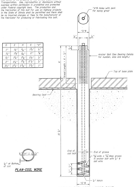
The Illinois Coil-Lock Anchor Bolt is a proprietary
