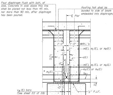
SECTION A-A AT ABUTMENT (at Rt. Ls)
