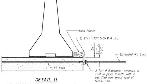
The 1"x7"x10" Plate shall not be removed until Stage II Construction forms and all reinforcement bars are in place and the concrete is ready to be
