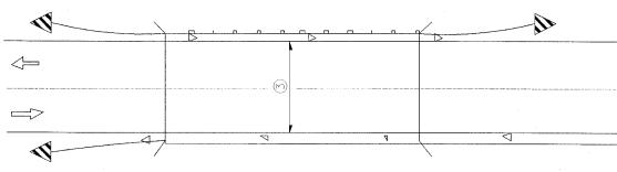
Bidirectional silver/silver should be used in lieu of monodirectional silver on both sides of two-lane bridges where the pavement is less than 24" wider than the pavement approaching the bridge.
