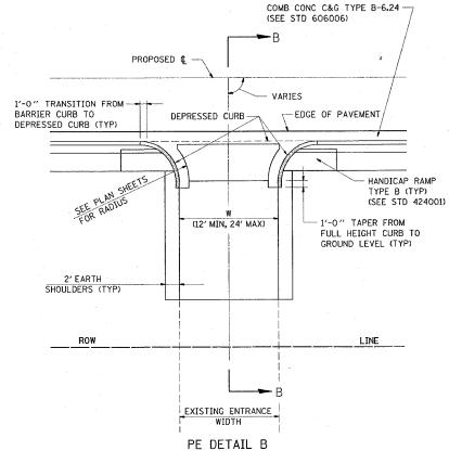
PRIVATE ENTRANCE WITH PCC SIDEWALK ADJACENT TO ROADWAY PAVEMENT WITH CONCRETE CURB & GUTTER TYPE 8-6.24
