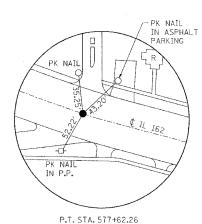
TBM 2020-2 CHISELED "□" ON N. CONC.FOUNDATION OF MOBIL GAS STATION SIGN @ SW QUADRANT OF IL 162 & I-55 ELEV = 570.497
