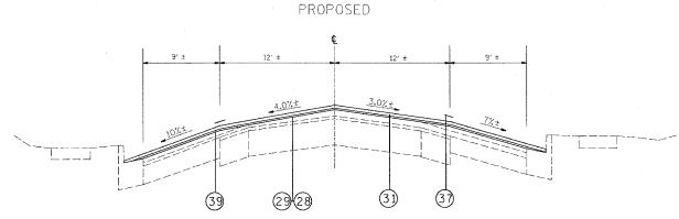
MILLING PROCEDURES: UTILIZE THE CENTERLINE FOR THE CONTROL POINT. MILL AT A ZERO DEPTH FROM THE CENTERLINE TO THE EDGE OF PAVEMENT, THIS SHOULD CREATE A 4% SLOPE ON THE LEFT AND A 3% SLOPE ON THE RIGHT. NO MILLING WILL BE DONE ON THE PARKING LANES. THIS WORK WILL BE PAID FOR AS (BITUMINOUS SURFACE REMOVAL (VARIABLE DEPTH)).
