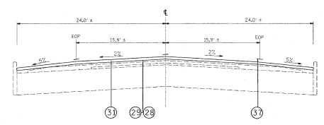
MILLING PROCEDURES: MILL  $1^{1}/2^{\circ}$  OF SURFACE USING THE CENTERLINE AS THE CONTROL POINT. MILL FROM THE CENTERLINE TO THE EDGE OF PAVEMENT AT A SLOPE OF 2%. THEN MILL  $1^{1}/2^{\circ}$  AT A RATE OF 5% FROM THE EDGE OF PAVEMENT TO THE CURB. THIS WORK WILL BE PAID FOR AS (BITUMINOUS SURFACE REMOVAL  $1^{1}/2^{\circ}$ ).
