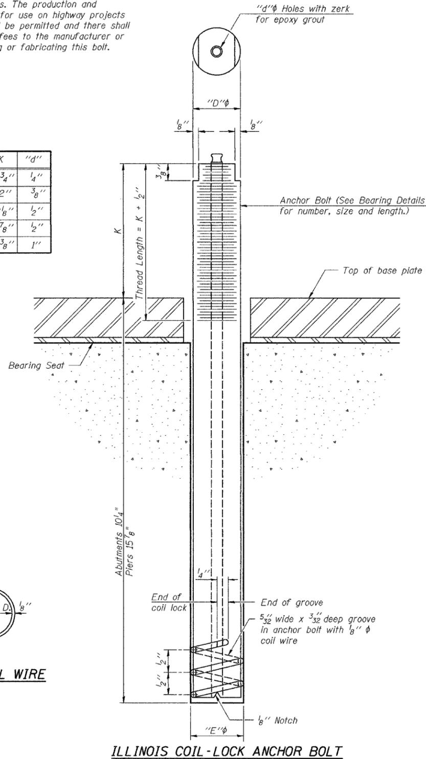
**MATERIALS FOR ILLINOIS COIL-LOCK ANCHOR BOLT**
