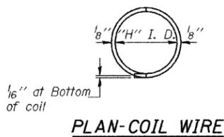
**ILLINOIS COIL-LOCK ANCHOR BOLT**
