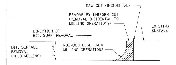
NOTE: WHEN MILLING OPERATIONS PRODUCE A ROUNDED EDGE, THEN A SAW CUT SHALL BE USED TO MANUFACTURE A PERPENDICULAR EDGE AS SHOWN IN THE DETAIL. THE ENGINEER SHALL BE THE SOLE JUDGE CONCERNING THE USE OF THIS DETAIL
