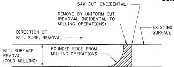
NOTE: WHEN MILLING OPERATIONS PRODUCE A ROUNDED EDGE,
