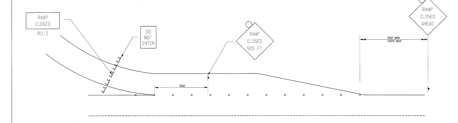
A CHECK BARRICADE SHALL BE PLACED IN THE MIDDLE OF THE CLOSED LANE AND AT THE SHOULDER AT 500' CENTERS
