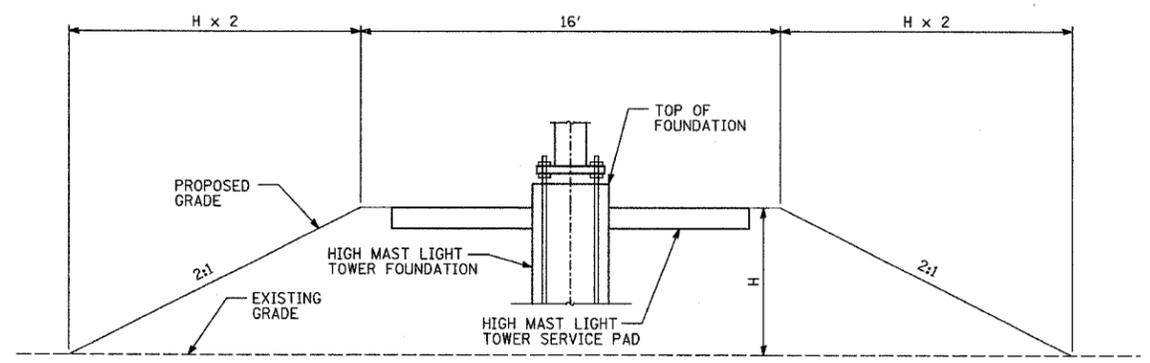
FILL GRADING DETAIL SECTION A-A
