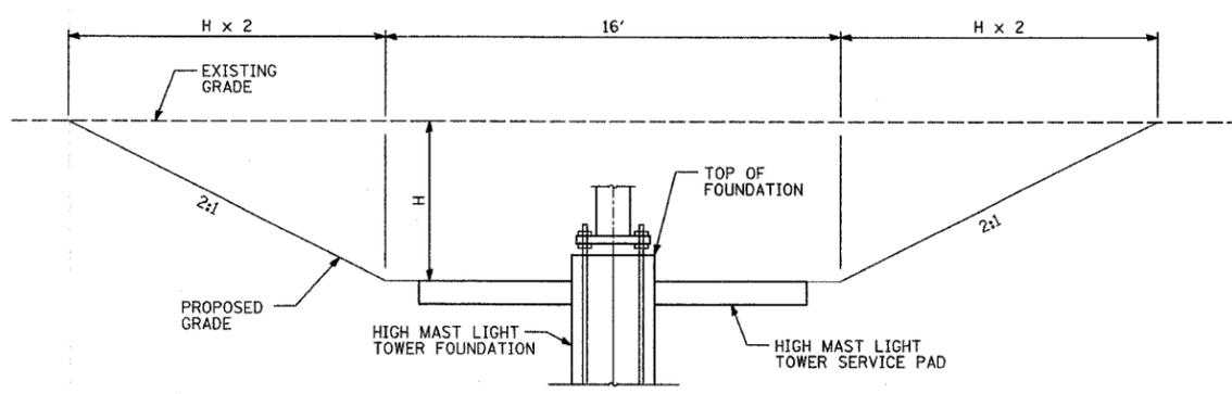
CUT GRADING DETAIL SECTION A-A
