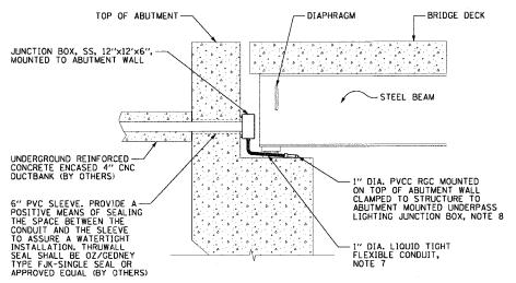
TYPICAL CONDUIT INSTALLATION THROUGH ABUTMENT WALL FOR LIGHTING SERVICE FEED ME-05F SCALE: 1/2" = 1'-0"
