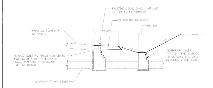
TEMPORARY INLET WHERE EXISTING STRUCTURE IS TO BE RELOCATED ALONG THE SAME EXISTING SEWER MAIN
