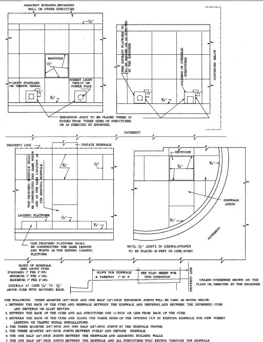
7. THE ONE HALF (12") INCH JOINTS BETWEEN THE SIDEWALK AND ALL STRUCTURES THAT EXTEND THROUGH THE SIDEWALK SUCH AS LIGHT STANDARDS, TROLLY, AND POWER POLES, COLUMNS, OF OVERHEAD STRUCTURES, MANHOLES, ETC.
