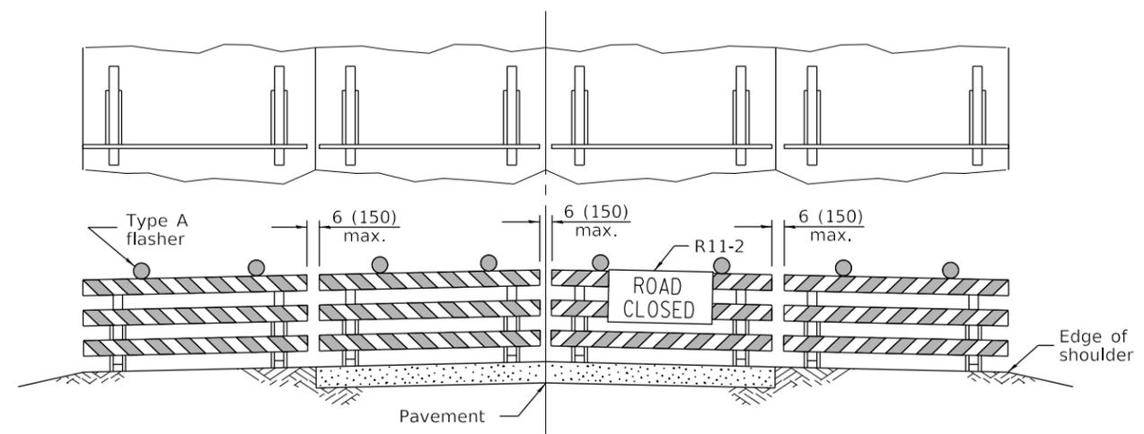
Reflectorized striping may be omitted on the back side of the barricades. If a Type III barricade with an attached sign panel which meets NCHRP 350 is not available, the sign may be mounted on an NCHRP 350 temporary sign support directly in front of the barricade.
