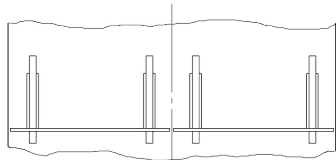
Type III Barricades with Standard Sign R11-2 or R11-4 mounted as shown.
