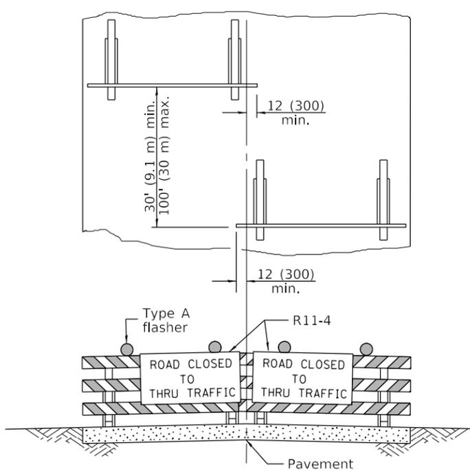
Reflectorized striping shall appear on both sides of the barricades. If a Type III barricade with an attached sign panel which meets NCHRP 350 is not available, the signs may be mounted on NCHRP 350 temporary sign supports directly in front of the barricade.
