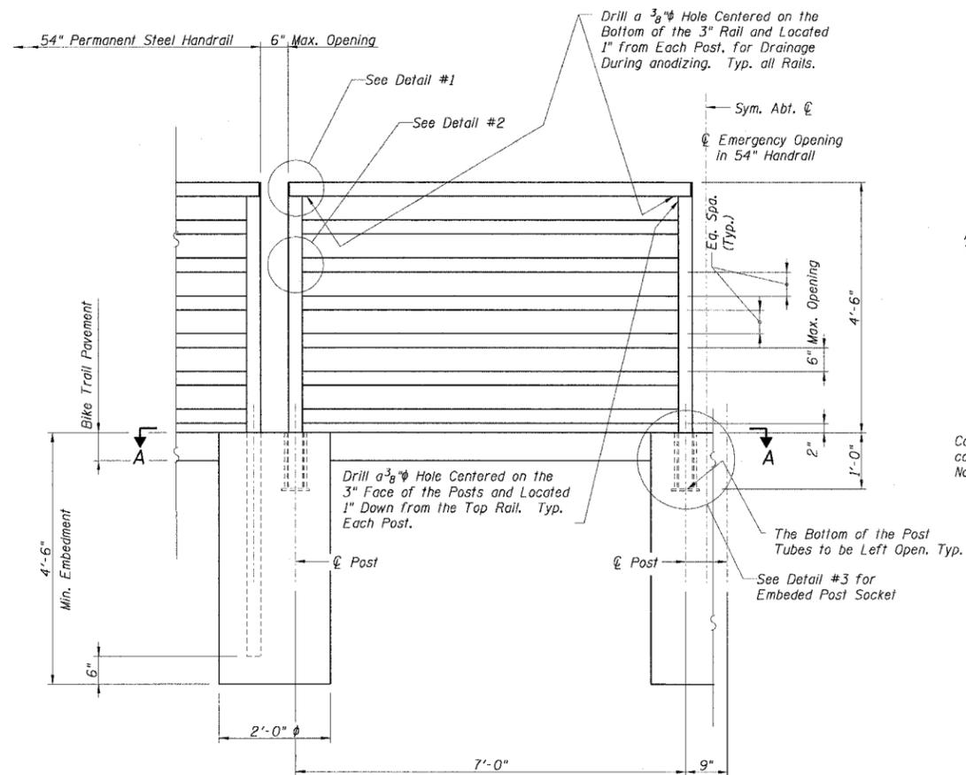
**PARTIAL ELEVATION - REMOVABLE HANDRAIL, 54"**
