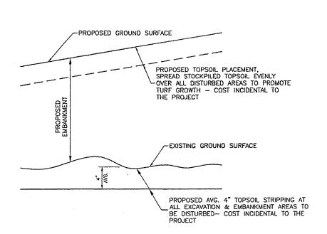
TOPSOIL STRIPPING DETAIL N.T.S.
