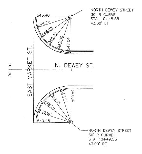
NOTE: ALL ELEVATIONS ARE GIVEN AT THE EDGE OF PAVEMENT.
