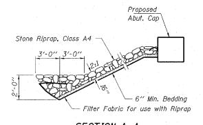
SECTION A-A Note: See Special Provisions for Stone Riprap, Class A4.
