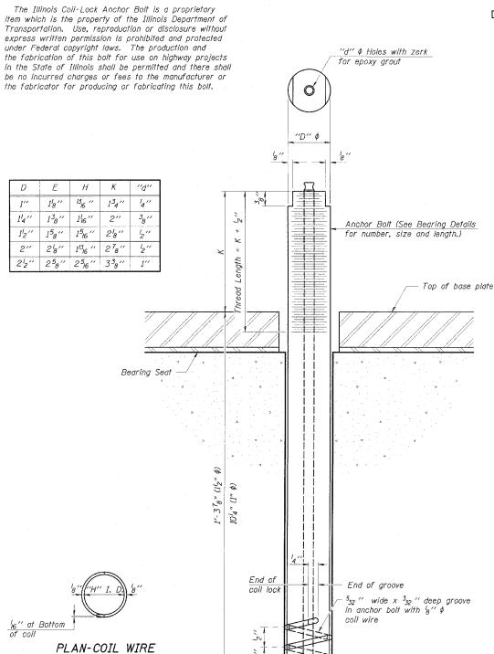
ILLINOIS COIL-LOCK ANCHOR BOLT
