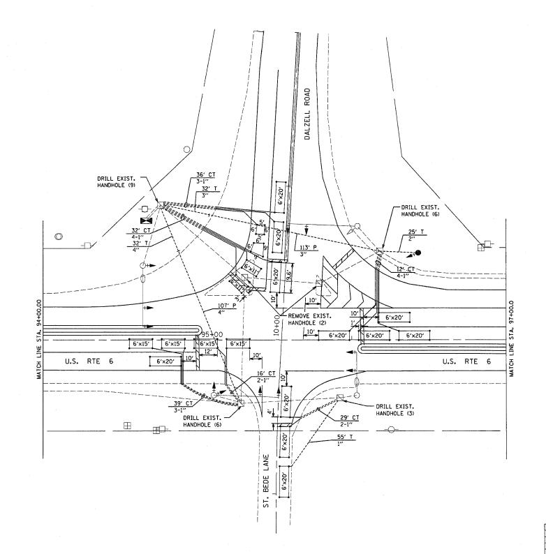
TRAFFIC SIGNALS LEGEND EXISTING PROPOSED  $\bowtie$ CONTROLLER CABINET CONDUIT \_\_\_\_\_ SIGNAL HEAD WITH BACKPLATE --> STEEL MAST ARM 0 TRAFFIC SIGNAL POST HANDHOLE
