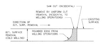
NOTE: WHEN MILLING OPERATIONS PRODUCE A ROUNDED EDGE,
