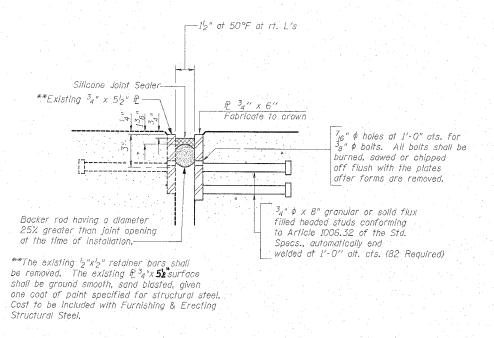
SECTION THRU EXPANSION JOINT @ N. ABT.
