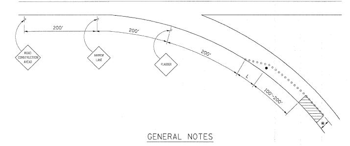
CONES AT 8 m (25')CENTERS FOR 105 m (350'). ADDITIONAL CONES MAY BE PLACED AT 15 m (50') CENTERS. WHEN DRUMS OR BARRICADES ARE USED. THE INTERVAL DEVICES MAY BE DOUBLED.
