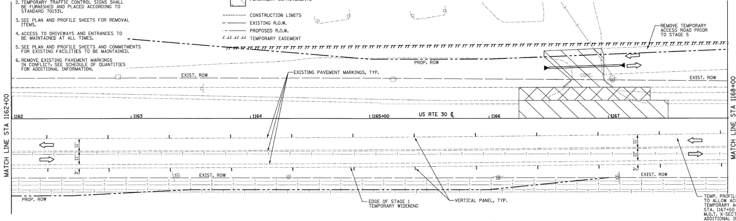
TEMP. PROFILE ADJUSTMENT, TO ALLOW ACCESS TO THE TEMPORARY ACCESS ROAD, STA. 1167+50 TO 1170+50. SEE M.O.T. X-SECTIONS FOR ADDITIONAL INFORMATION.
